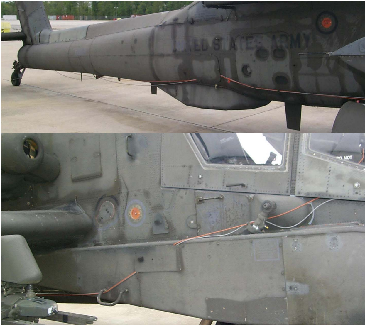
Figure 15. Tail Accelerometer Cable Routing
