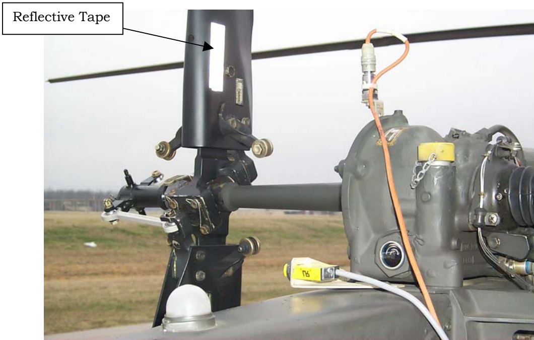
Figure 7. Reflective Tape Installation
